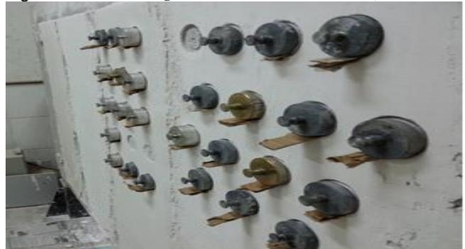
After waiting 24 hours for drying of the glue, it began the tearing of the specimens using the aderimeter (Figure 5).
