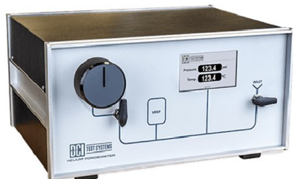
Figure 4. Helium Porosimeter at the Petrophysics Laboratory of the DEN-UFPE. Font: Veiga et al. (2024).
