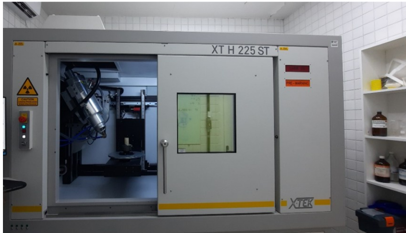
Figure 5. X-ray Computed Tomography Scanner at the DEN-UFPE. Font: Veiga et al. (2024).
