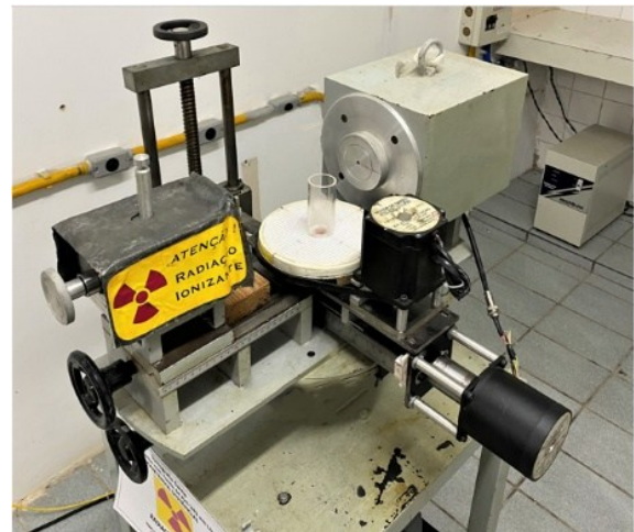
Figure 2. First-generation gamma-ray computed tomography scanner (TGC - 1st Gen) of the DEN at the UFPE. Font: Carvalho et al. (2024).
